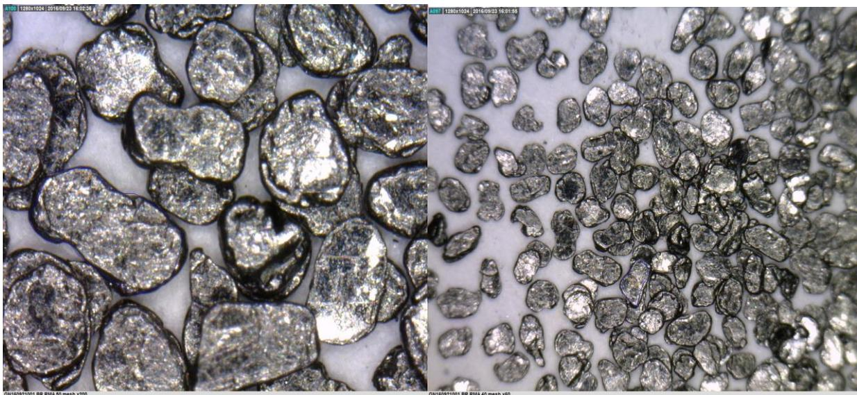
**Figure 2. Optical micrographs demonstrating thick, blocky graphite flakes**
