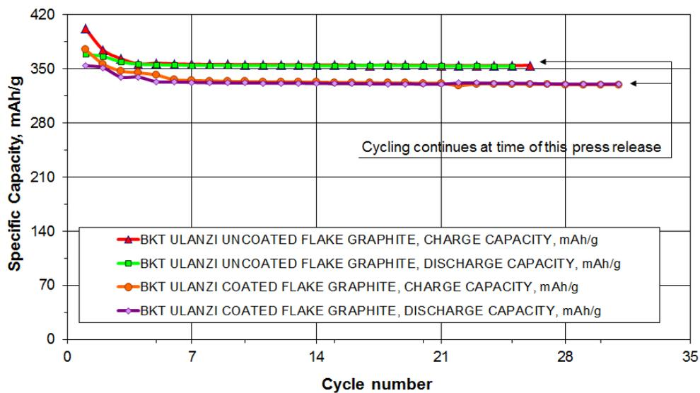
**Figure 7. Initial long-term cycling data with surface coated BKT Flake (sample BKT161206001) and uncoated BKT Flake (sample BKT161206004) at C/20 formation followed by C/10 cycling regime.**
