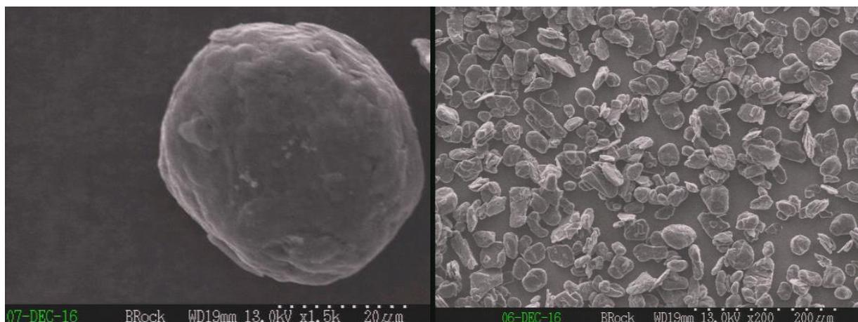
**Figure 1. SEM of surface coated spheroidal flake, BKT161206001.**
