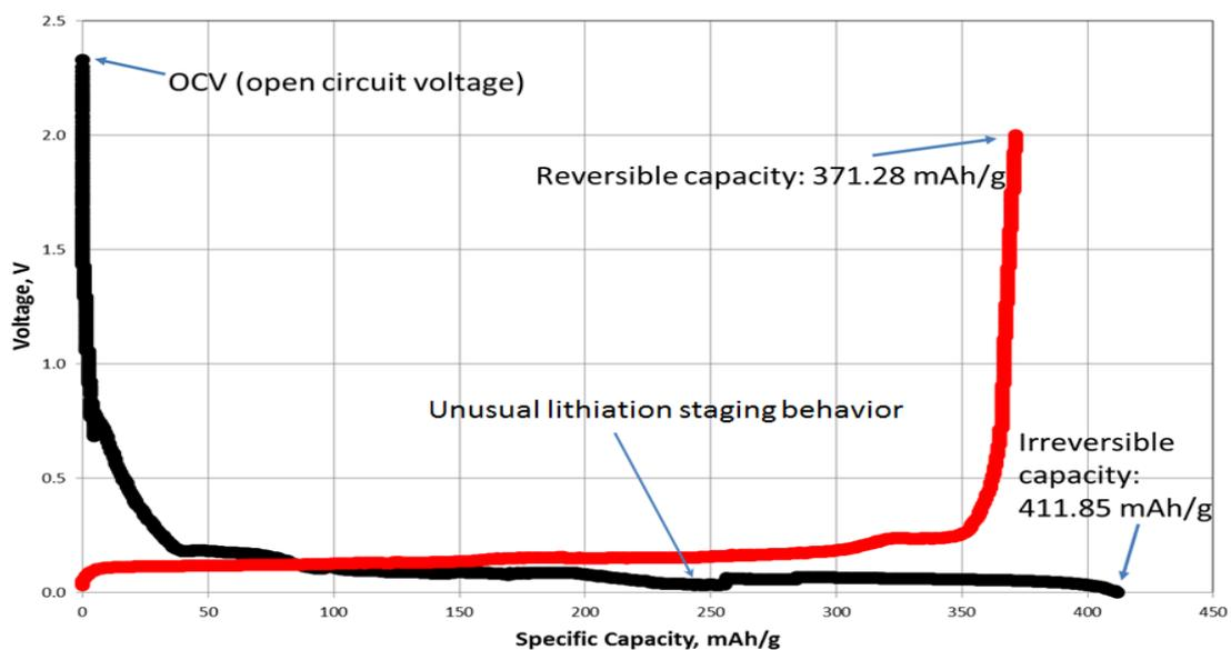
**Figure 4. Initial Galvanostatic Behavior of Uncoated BKT Flake (sample BKT161206004) in a CR2016 coin cell vs. Li/Li<sup>+</sup> counter electrode at an ultra-slow cycling rate of C/100.**
