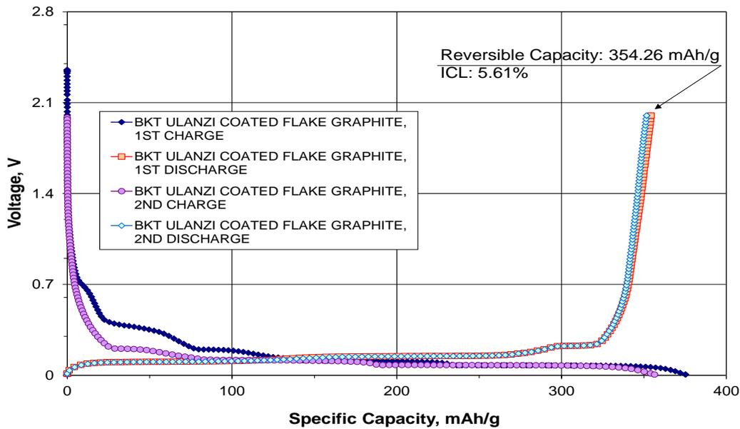
**Figure 6. Initial Galvanostatic Cycling of surface coated BKT Flake (sample BKT161206001) in a CR2016 coin cell vs. Li/Li<sup>+</sup> counter electrode at a cycling rate of C/20.**
