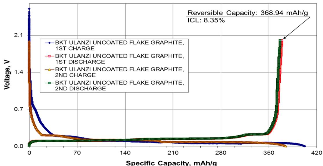
**Figure 5. Initial Galvanostatic Cycling of Uncoated BKT Flake (sample BKT161206004) in a CR2016 coin cell vs. Li/Li<sup>+</sup> counter electrode at a battery industry typical cycling rate of C/20.**
